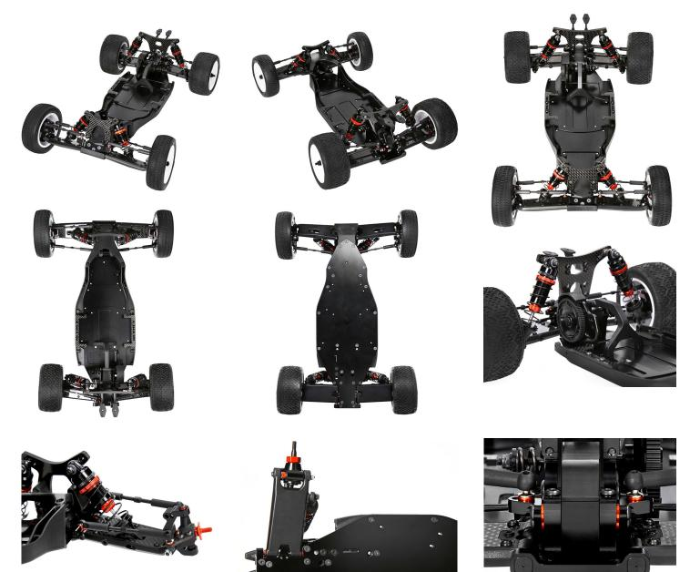
The D2 Evo is supplied in kit form. Requires body, wing, battery, motor, ESC, radio, receiver, servo, paint, tires, CA glue, wheels.
